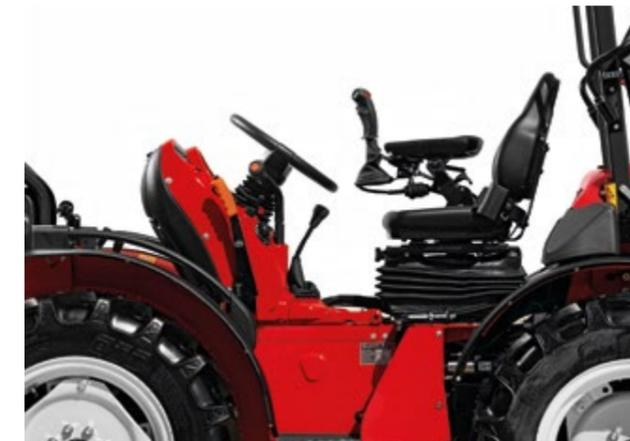
The spacious operator's platform thermally and acoustically isolates the cab from the transmission, providing comfort during operating and drastically reducing vibrations. The suspended pedal assembly of the RGS™ reversible driver's seat, an integral part of the rotating turret, has no gaps towards the ground, a feature that protects the driver's seat equipment and the operator from the entry of dust.
